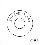
With the ignition switch ON, pushing this button at the right-hand drive station will perform the same function as turning the key to the START position at the left-hand drive station.
