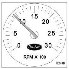
Your tachometer measures the engine speed in revolutions-perminute (RPM). Watching your tachometer is important to driving efficiently. It will let you match driving speed and gear selection to the operating range of your engine. If your engine speed gets too high, you can select a higher gear to lower the RPM. If your engine speed drops too low, you can select a lower gear to raise the RPM.
