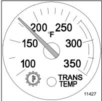
Your Transmission Temperature Gauge indicates the temperature of the oil in your transmission. Watch this gauge to know when your transmission is overheating. If it is, have it checked by an authorized service representative. Maximum transmission temperature may vary, depending upon the transmission and type of lubricant. It is typically 250° F (121° C); check your transmission's owner's manual.
