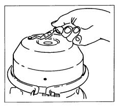
2. Remove the release stud assembly from the side pocket: remove the release nut and washer from the release stud.
