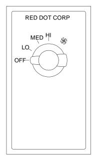
**To cool the cab,** turn on the air conditioning system and adjust the blower speed until comfortable. The amount of cooling is controlled by
