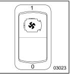
The engine fan switch allows you to control the engine fan manually or automatically. With the ignition key switch ON and the fan switch in the ON position, the engine fan will be on regardless of engine temperature. With the engine fan switch in the AUTOMATIC position, the
