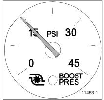
Your manifold pressure gauge indicates the power your engine is putting out by showing the amount of turbo boost. If the pressure indicated by your manifold pressure gauge goes down, there may be something wrong with your engine. Have it checked by a qualified service person.
