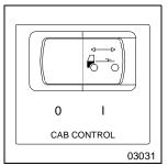
Vehicles having an air-slide fifth wheel have a fifth wheel slider lock controlled by a switch on the instrument panel. By placing the switch in the unlock position, you can slide the fifth wheel to various positions to adjust weight distribution.
