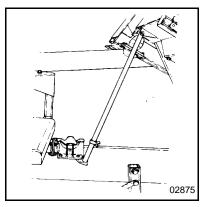
Locking Bar in Anchored Positioned
