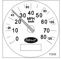
The speedometer-message center (SMC) is a combination of a speedometer and a message center. The speedometer indicates your vehicle's speed in both miles and kilometers per hour. The message center contains a 7-character, segmented LCD screen that can display the following items:
