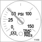
This gauge will show you how much air pressure is being applied from your foot brake valve or trailer brake hand valve.
