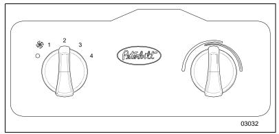
• **To heat the cab,** select the "Cab" mode and the desired air source, then adjust the air temperature lever and blower speed until comfortable.
