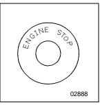
Pushing this button at the right-hand drive station stops the engine.
