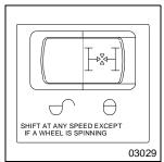
The interaxle differential allows differential action between the forward rear and the rear rear driving axles. The interaxle differential lock switch allows the operator to LOCK or UNLOCK the differential. There is a guard over this switch to prevent you from accidentally activating the lock.
