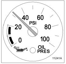
It is important to maintain oil pressure within acceptable limits. Your engine manual will give you normal operating pressures for your particular engine.
