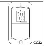
Mirror heat is controlled by the control panel switch shown above. If the vehicle is equipped with this switch, mirror heat can be switched on to help remove frost and ice from the mirror glass.
