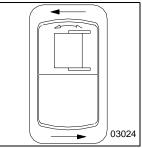
The power mirror control controls the adjustment of the right or left outside mirrors, depending on the option selected.
