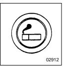
To operate your lighter, push the knob in. After a few moments the lighter will automatically pop out, ready to use. After use, insert the knob, but don't push it in. The lighter circuit is protected by a 20-ampere fuse to prevent damage should the lighter get stuck in the IN position. If this fuse needs replacement, check to ensure that the lighter is not stuck before replacing the fuse.
