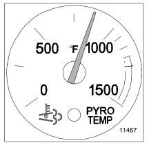
The pyrometer gauge indicates engine exhaust gas temperature. Since it responds almost immediately to changes in exhaust gas temperature, the pyrometer is an excellent indicator of engine output.
