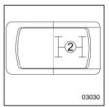
If your vehicle is equipped with a two-speed rear axle, you can select the axle range by the dash-mounted switch shown above. The low range provides maximum torque for operating off-highway. The high range is a faster ratio for highway speeds. There is a guard over this switch to prevent you from accidentally changing speeds.
