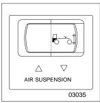
If your vehicle is a tractor with a rear air suspension, it may have an air suspension deflation switch on the dash that allows the air in the suspension to be exhausted. The purpose of this feature is to allow you to lower your tractor to get under a trailer.
