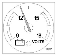
Your voltmeter displays the battery voltage. Normally, it should show 12V to 14V (volts).
