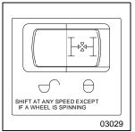
In the LOCK position, an air operated clutch positively locks both sets of axles together, providing greater traction on slippery road surfaces; however, steering around corners and on dry pavement is more difficult. Continuous operation on a paved, dry surface stresses the tandem axles, possibly causing internal damage to them.
