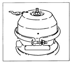
With a wrench, turn the release stud assembly nut until the compression spring is 90% - 95% caged. While doing this, check to make sure the push rod (adapter push rod or service push rod) is retracting. Do not overtorque the release stud assembly [S-Cam type maximum 50 Lb. ft. (68 N.m.); Wedge-type maximum 30 Lb. ft. (41 N.m.)]. The spring brake is now mechanically released.
