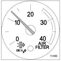
This gauge indicates the condition of the engine air cleaner and is measured by inches of water (H<sub>2</sub>O). A clean filter should register 7" H<sub>2</sub>O (may vary with system design); a filter whose life is over will register approximately 20" H<sub>2</sub>O (for Cummins engines) or 25" H<sub>2</sub>O (for Caterpillar engines).
