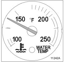
The water temperature gauge shows the temperature of the engine coolant. Under normal operating conditions the water temperature gauge should register between 165° and 210° - 225° F (99° and 107° C), depending on the engine. Under certain conditions, somewhat higher temperatures may be acceptable. But the maximum allowable temperature is 225° F (107° C) with the cooling system pressurized, except for certain special engines. Check your engine manual to be sure.
