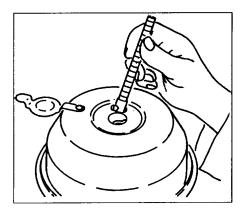
5. Assemble the release stud washer and nut on the release stud.
