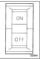
A two-position switch controls each dome light.
